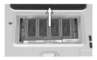
11 Hold the new or replacement module at a 30-degree angle and press it into the empty memory slot. This module is keyed so it can only be inserted in one direction. If the module does not fit, make sure that the notch in the module lines up with the tab in the memory bay.
